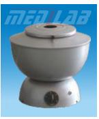
swing out rotor head with five step speed regulator, operates on 220-240V AC, 50Hz, maximum RPM 3600
