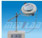
illuminated, glass lens dia. 145mm, magnification 2x, focal length 250mm.
