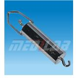
used to demonstrate Archimedes principle. It is a Brass cylinder with a suspension hook at one end in a close fitting Brass bucket with a handle and a hook on either side.
