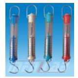
Acrylic, Tubular type, each range is color coded for easy identification, dual scale both in grams and Newton, provision for zero adjustment at top.
