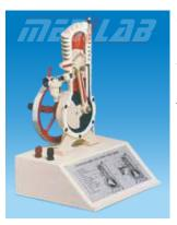
demonstrate operation of simple piston air cooled two stroke engine, mounted on a polished wooden base with schematic diagram.
