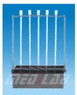
for demonstration of comparison of thermal and volumetric expansion of five different liquids. It has five glass bulbs with funnel shaped mouth, all supported by a metal frame.
