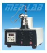
for accurate determination of melting points of solid samples. The unit consists of a built-in magnetic stirrer, an electrode controller for adjusting the rate of heating of silicon oil bath, ON/OFF switch, a pilot lamp, magnifier, a glare free illuminated background, a HIGH/LOW range selector switch and a digital temperature indicator with PT-100 sensor.
