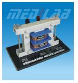
set of 3 coils-one main primary coil 240V, 2400 turns and two interchangeable secondary coils 65 turns and 130 turns, each giving output of about 6V and 12V respectively at a maximum current rating of 2A, with number of turns and current/voltage rating marked on each coil.
