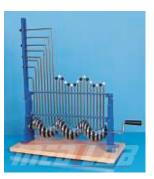
consists of 24 nos. aluminium disc supporting a series of iron-nickel rods. By revolving the handle, the motion is transmitted successively from one rod to the next, operating as a wave traveling to the top and back, by this, movement of waves can be observed.
