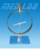
a metal ring frame of dia 12cm, carrying an insulating bush with a circular metal disc electrode on upper side. A light weight metal strip is pivoted at the center of ring to provide deflection with charging of electrode.
