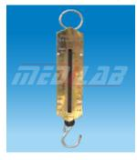
Brass, Flat form, painted metal case, provision for zero adjustment at the top.
