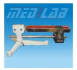
for producing vibrations in the stretched strings. An electromagnet operating on 6V is positioned between both the prongs and can slide along the length of the prong to adjust amplitude of vibrations. End of both prongs have a stylus for frequency measurement.
