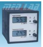
panel type, 96x96x110mm DIN size, calibration certificate optional Input: Capacitive RTD Range: 0 to 100% rH, -10 to 60° C Resolution: 0.1°rH, 0.1°C Accuracy:  $\pm 2\% \pm 1 \text{ digit} \pm 0.3^{\circ}\text{C}$
