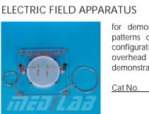
for demonstration of electric field patterns due to various electrodes configuration. It can also be placed on overhead projector to show the demonstration.
