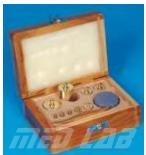
Polished Brass, knobed, nicely packed in a polished wooden box, also contains fractional weight box.
