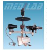
The principal elements of the assembly are: Specially designed Condenser, a light source and a measuring microscope. The microscope can be adjusted smoothly by slow motion screws in the horizontal as well as in the vertical direction. Automizer is also fitted on the same carriage. The apparatus does not need any critical adjustment and the oil drops appear in microscope within seconds. Microscope is provided with micro meter scale.
