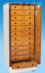
For keeping botanical specimens securely placed in herbarium sheets. Cabinet frame of 19 mm plyboard finished with laminated sheet. Hinged MDF baton to collectively lock the drawers. Drawer frame of MDF with plyboard bottom fitted with puller knobs and index card holder. Phosphor bronze clip provided inside drawer for keeping herbarium sheets in position. Drawers finished in spirit polish. Drawer Size 45cm x 37cm x 8cm.
