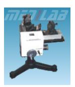
To determine the wavelength of Sodium Light/ Laser light using Michalson Interferometer with arrangement to micro measure highly polished plane slabs placed parallel at 45 and mirrors are placed at right angle. Laser light with power supply fitted. Fringes formed are easily visible on wall or paper.
