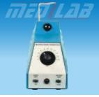
used in the determination of melting of any substance in small quantity upto 300°C.The apparatus is supplied with thermometer and capillaries, operates on 220-240V, 50Hz
