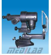
coincidence focusing system, 15x eyepieces, one position instrument, measure both meridians without changing optical system, the achromatic optical systems to precise measurement of the corneal radius curvature and accurate measurement of radius curvature of contact lens.
