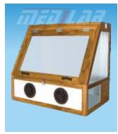
Made of seasoned teakwood with thick MDF sheet on top, bottom & back. Thick non-rattling glass provided on two sides and front slanting glass door. Front side slanting provided with openable glass door for convenient view of the specimens placed inside. Lower portion with round openings on front and one window on side. Inside painted white. Provided with one fluorescent tube and one U.V. tube. Nicely polished.
