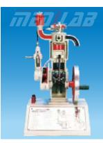
demonstrates functioning of fuel injection system together with hot coil starting device, mounted on a polished wooden base with schematic diagram.
