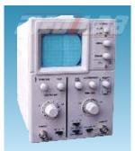
Fully solid state workable on 220 volts 50Hz. All supplies are established for accurate and stable operation. Single beam with a band width DC to 10 MHz. The accurate triggering of time base enable clear and stable display on screen 8x8cm. Vertical deflection can be selected for either A.C. or D.C. provision for attenuation in the input circuit, calibrated from 5mV to 50 V/cm.
