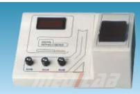
Features •Highly stable & accurate • Display – 31/2 digit LED • 30mm flat bottom Test Tube • Range 0 – 200 NTU Cat No. 13168
