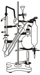
comprising of steam generation flask steam trap, vacuum jacketed flask with funnel, condenser tube of silver and receiving flask, complete with stand, clamp etc.
