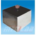
used for qualitative experiments of thermal radiation. This is a sheet metal cube of 13cm with opening at top to fill it with water.
