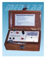
Direct reading of moisture in Timber, Pulp, Cotton wood. The instrument is housed in cabinet highly finished the test procedure is written on the panel, complete with probe and battery.
